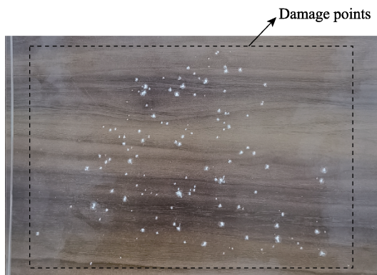
图 1 含损伤点熔石英玻璃真空窗口光学元件照片 Fig. 1 Photo of optical elements with damage points in the fused silica glass vacuum window
