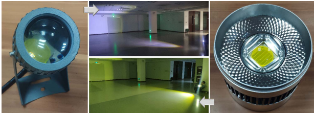
Fig. 11 Packaged LEDs devices from blue to yellow arbitrarily by adjusting the \text{Ce}^{3+} concentration and the thickness of transparent ceramics
