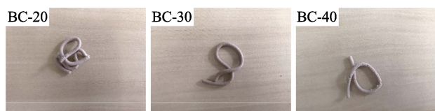
Fig. 8 Photographs of the mesoporous borosilicate bone cement extruded from the syringe
