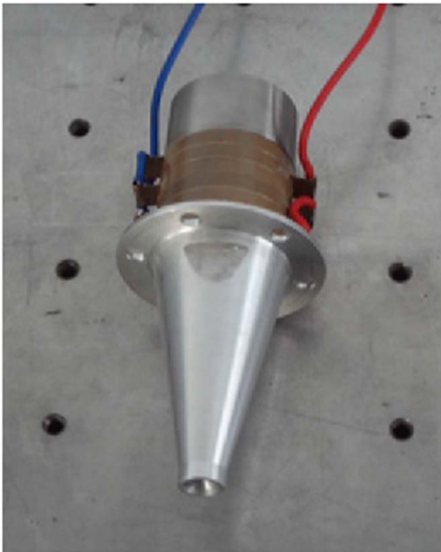
Figure 11. Photograph of the transducer with concave spherical surface: Liu et al [113]. [113] © The Korean Society of Mechanical Engineers and Springer-Verlag Berlin Heidelberg 2013. With permission of Springer.
