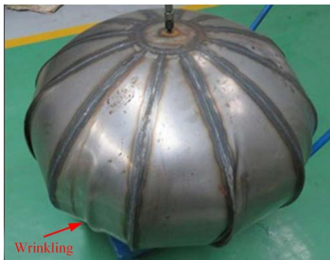
Figure 15. Severe wrinkling on ellipsoidal shell with initial axis length ratio of 2.2.
