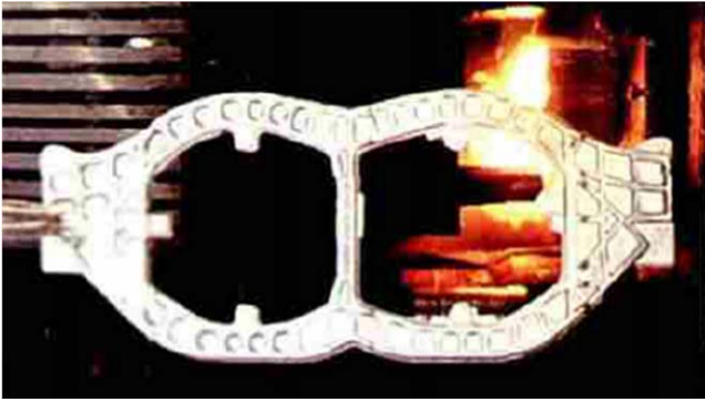
Figure 27. An integral titanium alloy frame with a 3.8 m width and 1.7 m height. Reproduced with permission from [75].
