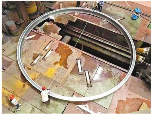
Figure 24. A 10 m diameter aluminum alloy ring. Reproduced with permission from [67].
