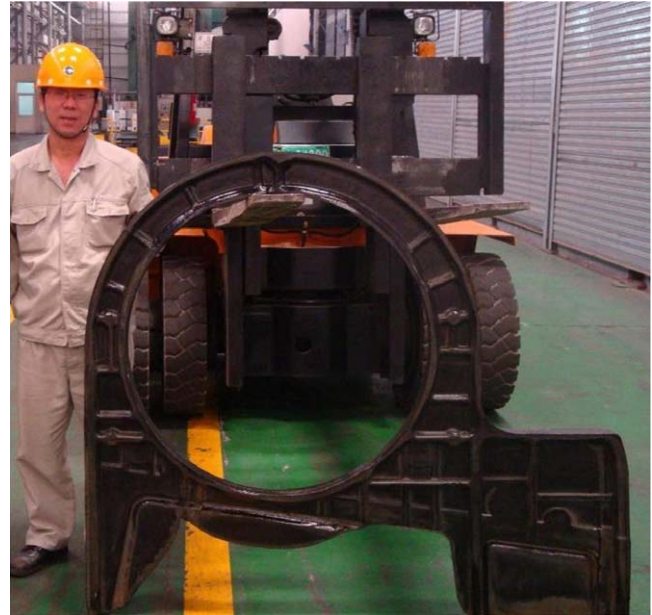
Figure 29. An integral titanium alloy rib-web component with projection area of 2 m 2 formed by a local isothermal forging process.
