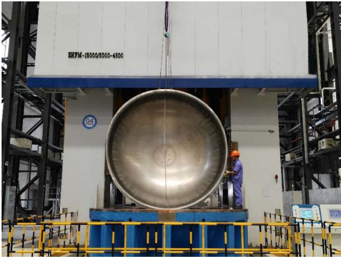
Figure 10. Aluminum alloy tank dome with 3 m in diameter and hydroforming press with 150 MN in drawing force and 5 m 3 in high pressure liquid volume.
