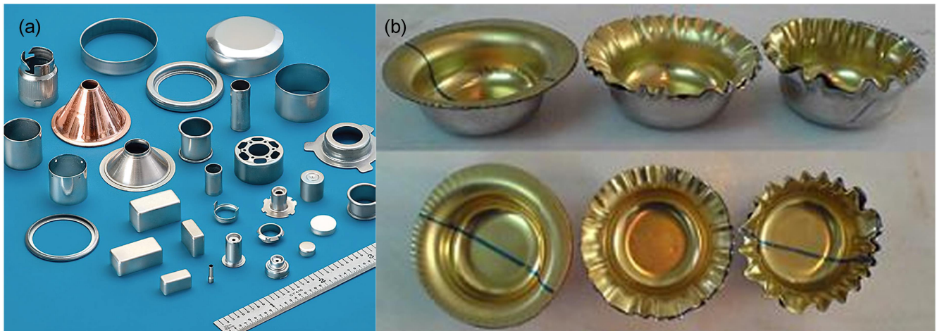
Figure 2. Miniature components produced by microforming: (a) microformed parts of various shapes [74] and (b) microdeep drawn parts of brass and steel [75]. (a) Reproduced with permission from [74]. (b) Reprinted from [75], Copyright (2013), with permission from Elsevier.
