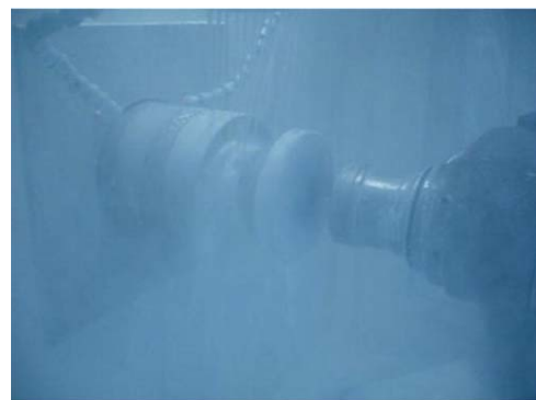
Figure 9. Fluid jet polishing.
