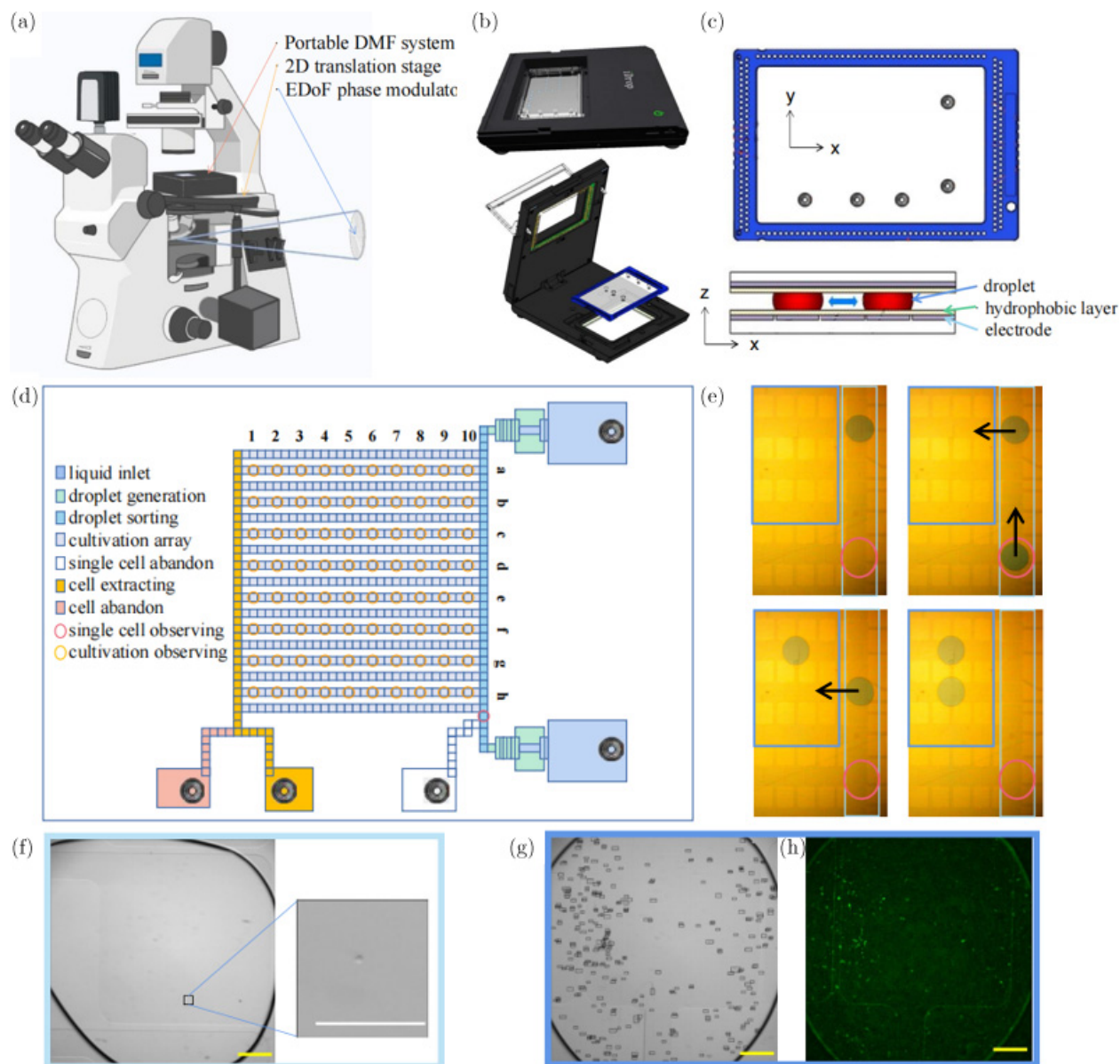
Fig. 2. The simple description of the DMF system. (a) The microscope equipped with the portable DMF system, a 2D translation stage, and the EDoF phase modulator. (b) The portable DMF system including the host and the chip, is mounted on the 2D translation platform. (c) The chip for manipulating the droplets. (d) The scheme of the chip with different function arrays. (e) The droplets can be controlled by the electrodes integrated on the chip, with the direction of movement indicated by the arrows, and recorded by microscope imaging. (f) The droplet containing a single yeast cell (see the inset) is observed. (g) The single yeast cell is cultured in the array for 36 h and this array is observed continuously. Each box represents a yeast cell at 36 h in the bright-field image. (h) The fluorescence image is obtained at 36 h to estimate the production of GFP. Scale bar: 200 \mu\text{m} .
