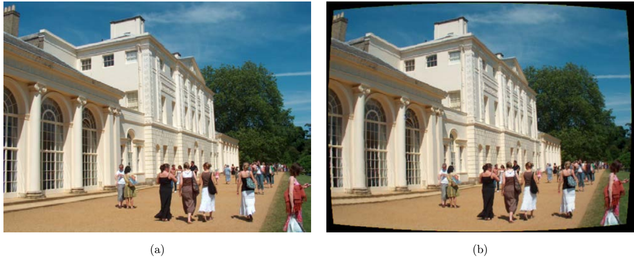
Fig. 16. The simulated result of the video endoscope system. (a) The original picture of object. (b) The picture imaged by the system.
