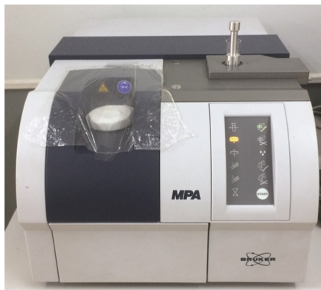
Fig. 1. Syrup spectra measurement by FT-NIR spectrometer.
