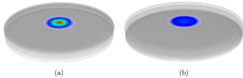
Fig. 3. Simulation results of the MOSE in the multilayered phantom. (a) Diffuse reflectance and (b) Transmittance.
