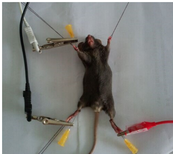
Fig. 3. ECG detection: The experiment use the BIOPAC multi-channel physiological recorder to collect the mouse's electrocardiogram signal, the electrode connection method: VIN+ connects the mouse's left leg, VIN- connects the mouse's right upper limb, GND connects the mouse's right leg.
