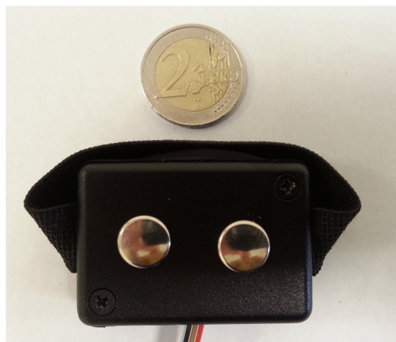
Fig. 5. Skin conductance sensor.
