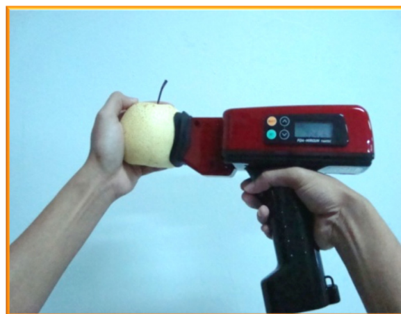
Fig. 1. The measuring of NIR spectrum on a pear in reflection mode using FQA-NIRGUN (Fantec, Japan).
