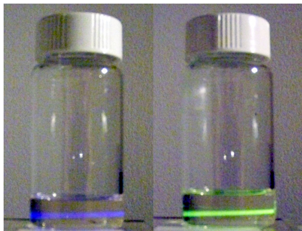
Fig. 1. NaYF 4 nanocrystals codoped with Yb 3+ and Tm 3+ (left) or Er 3+ (right). UCNP shown here were synthesized by thermal decomposition of LnTFA precursors, and had an average diameter of ~15 nm. Illumination was by laser diode at 980 nm.
