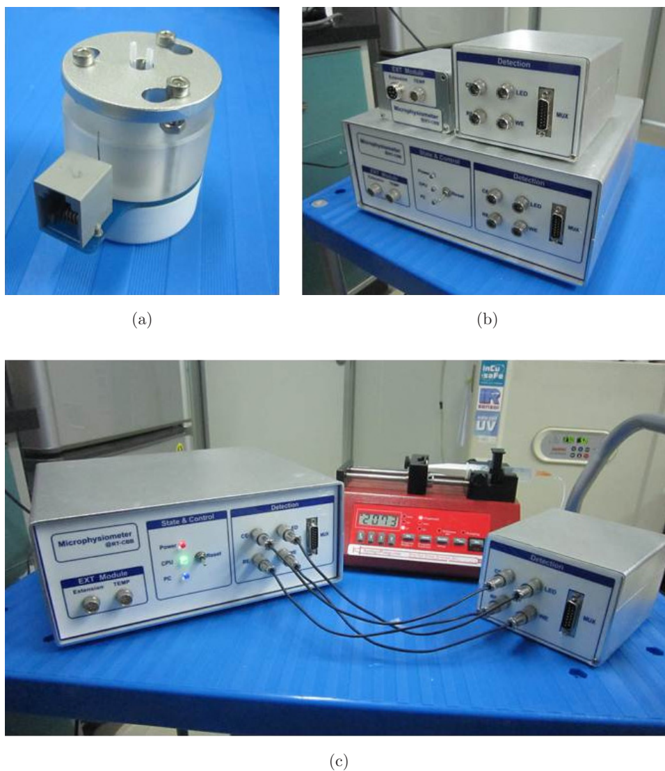
Fig. 4. The microphysiometer sensor unit and the system. (a) Microphysiometer sensor unit for cell culture with flow structure. (b) Microphysiometer system includes the core control and detecting instrument, sensor unit house and calibration box. (c) The whole microphysiometer detection system.
