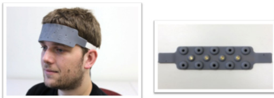
Fig. 4. Current version of the fNIR probe with a flexible circuit board and a cushioning, customized silicone material.
