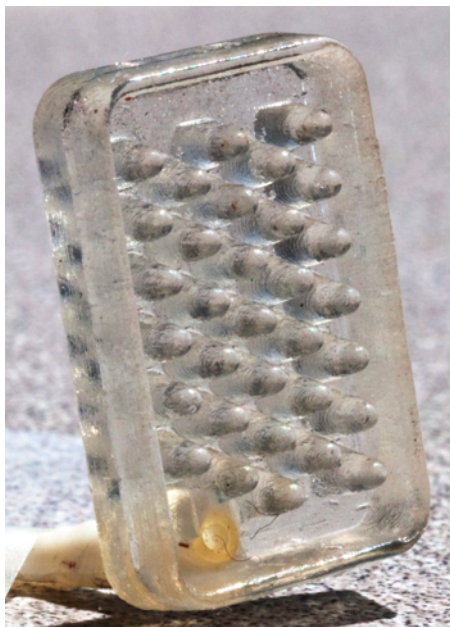
Fig. 1. Prototypical TOCD made using stereolithography. A 10 mm × 17 mm chamber is filled with an array of pins. A tube is connected to the chamber to apply vacuum pressure when a seal is formed while in contact with the tissue surface.
