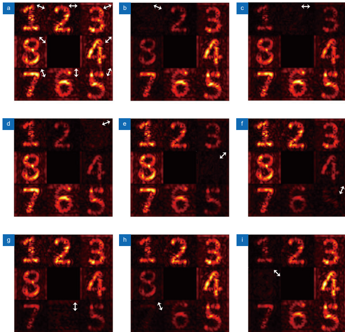
Fig. 5 | Experimental results for the image-hiding device. (a) Amplitude distribution of a hologram with no polarization state selected for detection. (b–i) Amplitude distributions when an image is hidden in channels C1 to C8, respectively, with the detected polarizations chosen as 67.5°, 90°, 112.5°, 135°, 157.5°, 0°, 22.5°, and 45°, respectively. Each white arrow represents the designed polarization state of the corresponding channel.
