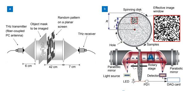
**Fig. 2** | (a) Single-pixel imaging system based on metallic binary masks for THz modulation<sup>43</sup>. (b) Spinning-disk based THz imaging setup. Figure reproduced from: (a) Ref.<sup>43</sup>, AIP Publishing; (b) Ref.<sup>44</sup>, Optical Society of America.
