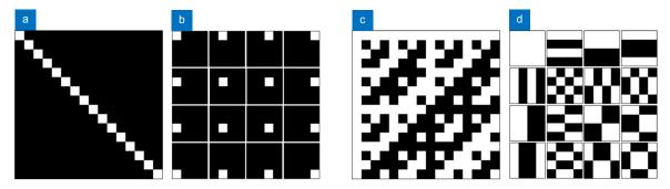
Fig. 1 | (a) 16 × 16 identity matrix H and (b) the corresponding series of 16 ( $n^2$ ), 4 × 4 spatial masks { $H_i(x,y)$ }<sub>i=1...16</sub> obtained from it; (c) 16 × 16 Hadamard matrix H and (d) corresponding set of 16, 4 × 4 spatial masks { $H_i(x,y)$ }<sub>i=1...16</sub>.
