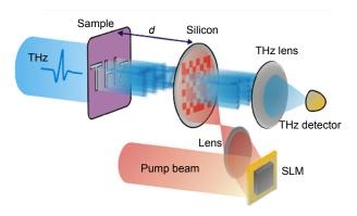
**Fig. 3 | All-optical modulation of a THz beam.** The patterning pump beam (visible/infrared) is modulated by an SLM. Subsequently, it illuminates the surface of a silicon plate and generates photo-carriers which transfer the pattern to the THz beam. Figure reproduced from Ref.<sup>62</sup>, Optical Society of America.
