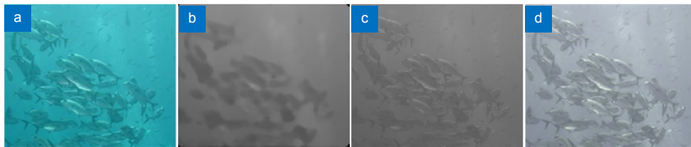
Fig. 5 | (a) Original image. (b) Red channel after compensation. (c) Red channel after guided filtering. (d) New RGB image.
