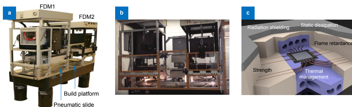
Fig. 1 | (a, b) Photograph of the multi 3D system. (c) Schematic of a fabrication example 9,14 . Figure reproduced from: (a) ref. 9 , Springer International Publishing AG; (b) ref. 14 , Elsevier Ltd; (c) ref. 9 , Springer International Publishing AG.
