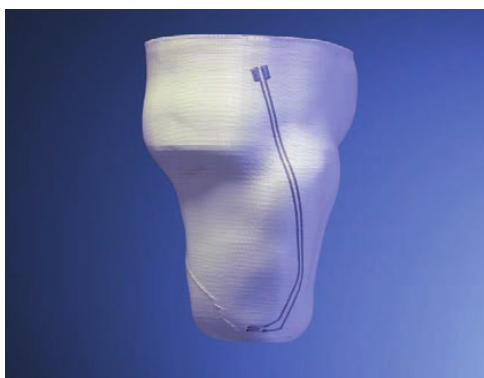
Fig. 12 | Leg prosthesis part produced by FDM and Aerosol Jet printing 31 . Figure reproduced from ref. 31 , University of Applied Science Bremerhaven.
