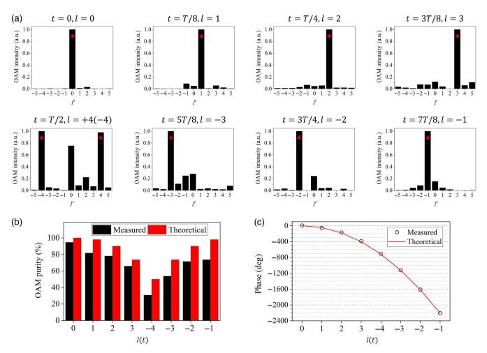
**Fig. 4** Spectrum analysis of time-varying OAM. (a) OAM intensity and phase spectrum of the measured time-varying OAM beams at different instants of time. (b) Measured and theoretical OAM mode purity for the dominant I(t). (c) Comparison of measured and theoretical twisting phases for different time instants of dominant I(t).
