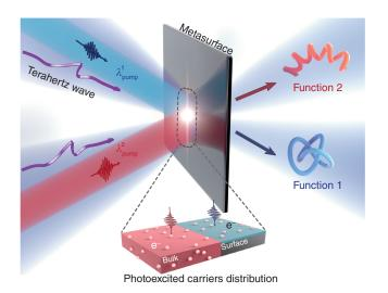
Fig. 1 Schematic of the dynamic dual-mode modulation with an optically controlled dielectric metasurface. Under pumping by external light at different wavelengths, a predesigned dielectric metasurface can exhibit distinct functionalities to manipulate THz waves.
