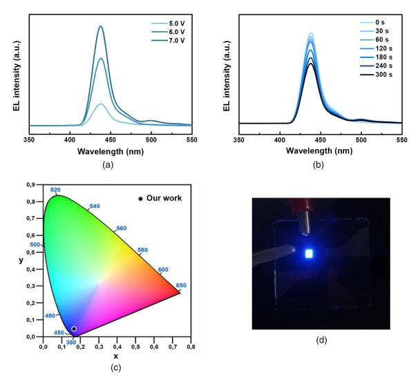
**Fig. 5** Stability of PeLEDs prepared from rapidly crystallized 2D perovskite films. (a) EL spectra as a function of bias voltage from 5 to 7 V. (b) EL spectra as a function of operation time. The intensities of the EL spectra negligibly changed under continuous operation for 5 min. (c) CIE 1931 chromatic coordinates and (d) digital photograph of the operating device.
