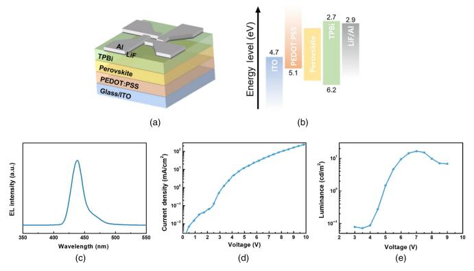
**Fig. 4** (a) Device configuration schematic and (b) band energy alignment of the PeLEDs. EL properties of PeLEDs fabricated from rapidly crystallized 2D perovskite films. (c) EL spectrum under a bias voltage of 6 V. (d) J - V and (e) L - V characteristics.
