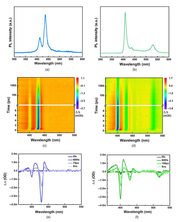
**Fig. 2** Steady-state PL spectra of 2D-RPP films fabricated by (a) rapid crystallization and (b) conventional hot-casting approaches on glass/ITO. TA mapping of (c) rapidly crystallized and (d) conventional hot-cast 2D-RPP films with respect to time delays. TA spectra at different time delays of the (e) rapidly crystallized and (f) conventional hot-cast 2D-RPP films.
