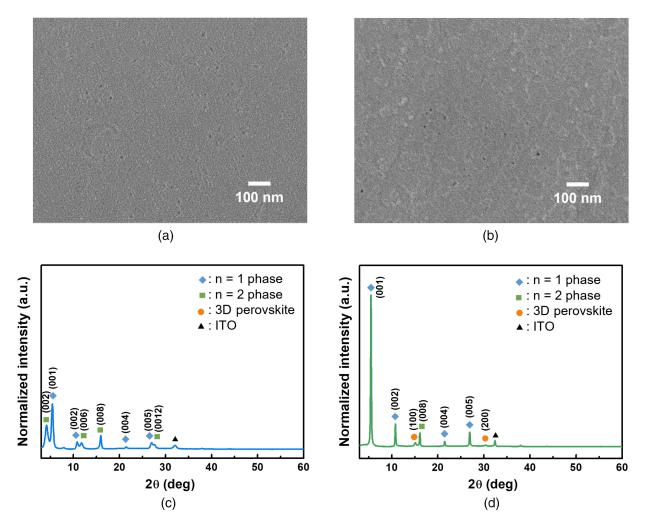
**Fig. 1** Top-view SEM images of (a) rapidly crystallized and (b) conventional hot-cast 2D perovskite films. XRD patterns of 2D-RPP films fabricated with (c) rapid crystallization and (d) conventional hot-casting methods on glass/ITO/PEDOT:PSS (the scale of the *y* axis was adjusted identically for both XRD spectra).
