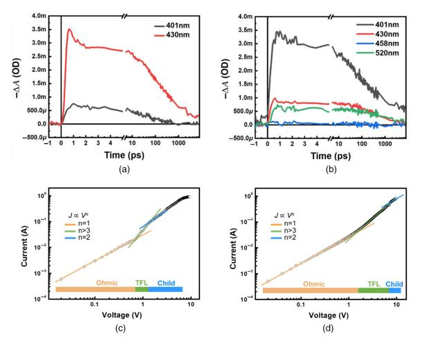
**Fig. 3** TA kinetics of the (a) rapidly crystallized and (b) conventional hot-cast 2D perovskite films probed at different wavelengths as a function of decay time. Current–voltage curves of hole-only devices fabricated from (c) rapidly crystallized and (d) conventional hot-cast 2D-RPP films obtained under dark conditions using the SCLC method. Hole-only devices in a configuration of glass/ITO/PEDOT:PSS/2D-RPPs/PTAA/AI were utilized.
