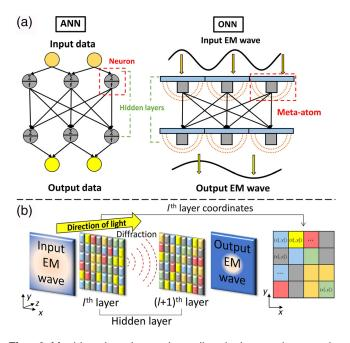
**Fig. 6** Machine learning using all-optical neural networks. (a) Comparison of the correspondence between ANNs and ONNs. The ANN is made up of neurons and hidden layers, which relate to the physical meta-atoms and cascaded metasurfaces in ONNs. (b) The coordinate system required to design ONNs using diffraction.
