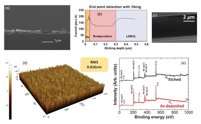
**Fig. 5** Dry etching results of LN. (a) SEM image of the LN cross section and (b) current changed along etching depth in end point detection after SF<sub>6</sub> based etching. (a) and (b) Adapted from Ref. 182 © 2008 American Institute of Physics (AIP). (c) SEM, (d) AFM, and (e) XPS images of LN sample after Ar-based dry etching. (c)–(e) Adapted with permission from Ref. 175.
