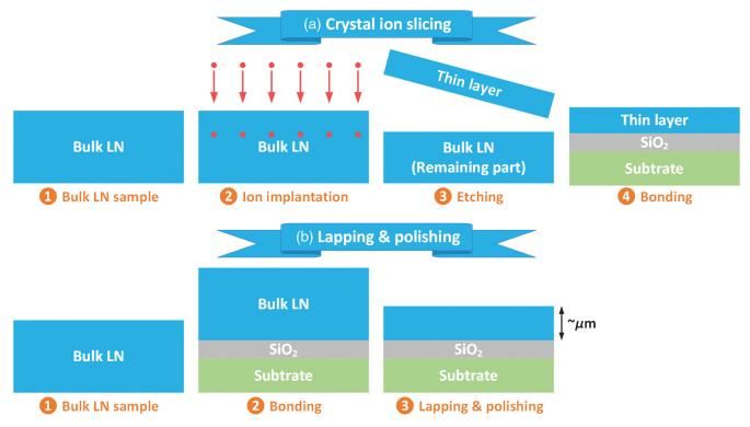
Fig. 3 Process flows of (a) CIS and (b) lapping and polishing technologies. Dimensions are not drawn to scale.
