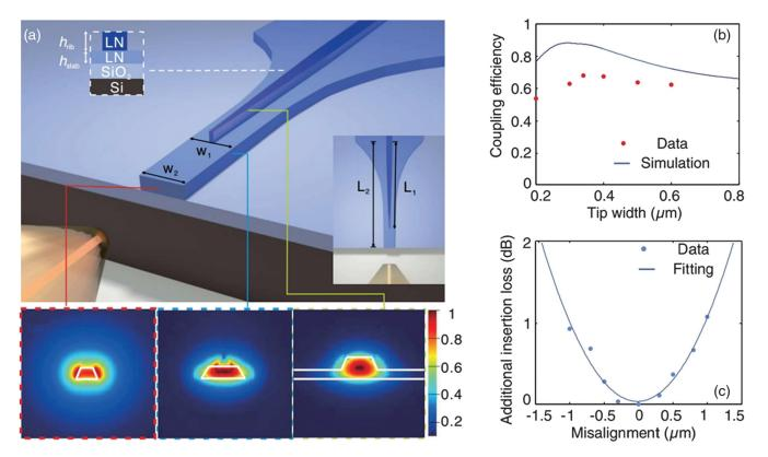
**Fig. 9** LN-based edge coupler. (a) Schematic structure of the bilayer edge coupler and its corresponding mode profiles at different positions. (b) Simulated and measured coupling efficiency versus different tip widths in the tapered slab region. (c) Additional insertion loss with respect to coupling misalignment (TE mode). (a)–(c) Adapted with permission from Ref. 246 © 2019 OSA.
