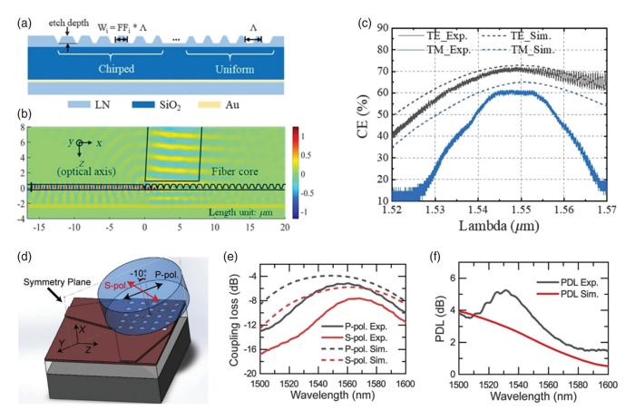
**Fig. 8** LN-based GCs. (a) Schematic structure, (b) simulated electric field distribution and (c) measured transmission spectrum of 1D chirped GC in TFLN. (a)–(c) Adapted with permission from Ref. 259 © 2020 OSA. (d) Schematic structure of a 2D GC in TFLN. Measured and simulated (e) transmission spectra and (f) polarization dependence loss of the TFLN 2D GC. (d)–(f) Adapted with permission from Ref. 265 © 2021 OSA.
