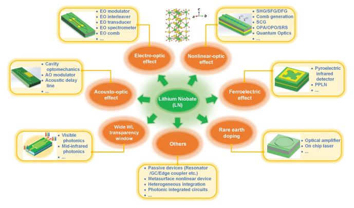
**Fig. 1** Overview of LN photonics. Top middle inset is LN crystal structure. EO, electro-optic; SHG, second harmonic generation; SFG/DFG, sum/difference frequency generation; SCG, supercontinuum generation; OPA/OPO, optical parametric amplification/oscillation; SRS, stimulated Raman scattering; PPLN, periodically poled lithium niobate; GC, grating coupler; WL, wavelength; AO, acousto-optic.
