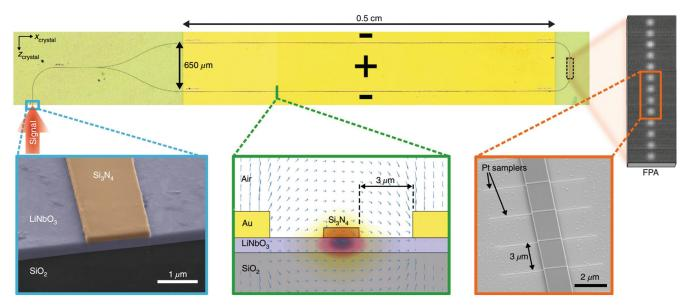
**Fig. 15** EO waveguide spectrometer in TFLN. Microscopic image and device details of an EO TFLN waveguide spectrometer. Adapted with permission from Ref. 171 © The Author(s), under exclusive license to SNL 2019.
