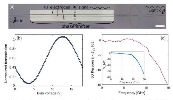
**Fig. 24** TFLN modulator operated at visible wavelength range. (a) Microscopic image of the TFLN EO modulator. (b) Measured transmission spectrum and (c)  $S_{21}$  curve. (a)–(c) Adapted with permission from Ref. 42 © 2019 OSA.
