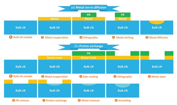
**Fig. 2** Process flow of planar LN device fabrication. Illustration of (a) metal ion-in diffusion and (b) PE methods for planar photonic device fabrication in bulk LN crystals (dimensions are not drawn to scale). PR, photoresist.
