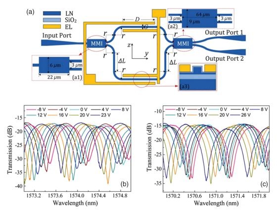
**Fig. 12** EO tunable interleaver in TFLN. (a) Schematic structure of TFLN waveguide interleaver, and its measured tunable transmission spectra for (b) TE and (c) TM polarized input light. (a)–(c) Adapted with permission from Ref. 297 © 2018 OSA.
