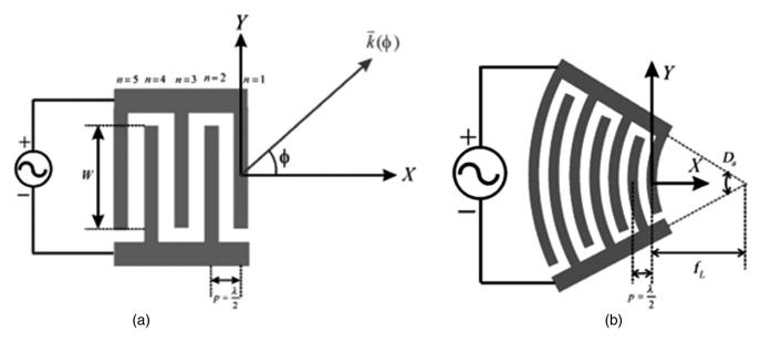
Fig. 18 Design of IDTs. Schematics of (a) straight and (b) concentric IDTs. (a) and (b) Adapted with permission from Ref. 315 © 2005 IEEE.
