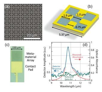
**Fig. 22** TFLN-based pyroelectric infrared detector. (a) SEM image of the metamaterial top surface. (b) Schematic of the unit cell. (c) Microscopic image of the pyroelectric PD. (d) Measured detector response and optical absorption of pyroelectric PD with and without metamaterial structure. (a)–(d) Adapted with permission from Ref. 18 © 2017 OSA.
