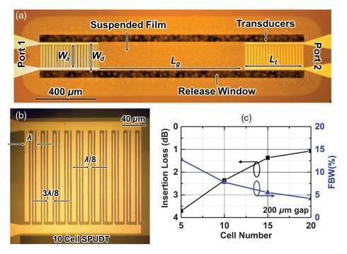
**Fig. 20** LN-based ADL. (a) Microscopic image of the fabricated ADL. (b) Microscopic image of zoomed in view of the device. (c) Extracted IL and FBW of ADLs with respect to cell numbers. (a)–(c) Adapted with permission from Ref. 321 © 2018 IEEE.
