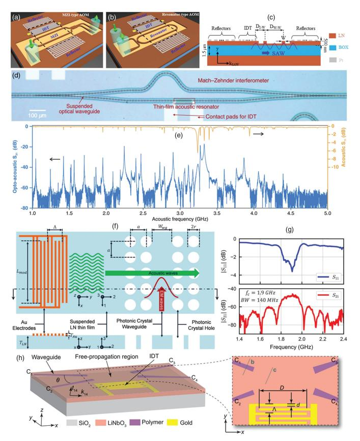
**Fig. 19** LN-based AO modulators. Schematics of (a) MZI and (b) microring type AO modulators. (c) Cross section of the AO modulator. (a)–(c) Adapted with permission from Ref. 16 © 2019 Chinese Laser Press (CLP). (d) Microscopic image of a suspended AO MZI. (e)  $S_{11}$  and  $S_{21}$  spectra of microwave to optical conversion. The optical power detected by photodetector (PD) is
