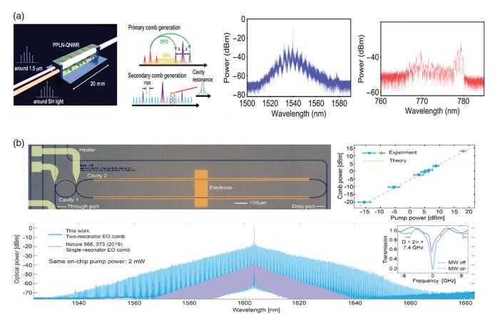
**Fig. 6** Using second-order nonlinear processes for generating OFCs on lithium niobate. (a) Quadratic frequency comb generation on conventional LN<sup>143</sup> using cascaded  $\chi^{(2)}$  processes, which has yet to be demonstrated on the TFLN platform. (b) Electro-optic frequency comb generation in TFLN using coupled microring and racetrack resonators and the resulting spectrum exhibiting a high conversion efficiency.<sup>148</sup>
