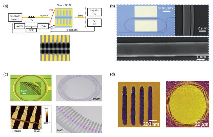
**Fig. 4** PPLN devices in different structures. (a) Straight waveguide.<sup>82</sup> (b) Racetrack resonator that is poled on one of the straight arms.<sup>83</sup> (c) Radially poled microring resonator.<sup>84</sup> (d) Radially poled microdisk, poled using the PFM technique in which they also demonstrated a poling period as small as 200 nm.<sup>85</sup>
