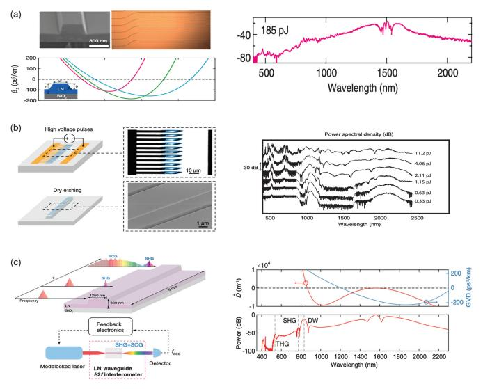
**Fig. 7** SCG on the TFLN platform. (a) SCG spanning over two octaves in a dispersion engineered straight waveguide without poling.<sup>159</sup> (b) SCG on a periodically poled straight waveguide with a span of more than two octaves at a pulse energy of ~11 pJ.<sup>139</sup> (c) Using cascaded SCG and SHG for on-chip f - 2f self-referencing, which is of great importance for realization of on-chip OFCs.<sup>158</sup>
