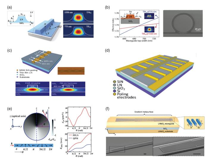
**Fig. 3** Various phase-matching methods used on the TFLN platform. (a) Birefringent phasematching.<sup>59</sup> (b) Modal phase matching.<sup>60</sup> (c) Grating-assisted quasi phase matching or mode shape modulation.<sup>61</sup> (d) PPLN on a straight waveguide.<sup>13</sup> (e) Natural quasi phase matching, which is conceptually similar to cyclic phase-matching.<sup>62</sup> (f) Phase-matching-free metasurface.<sup>63</sup>
