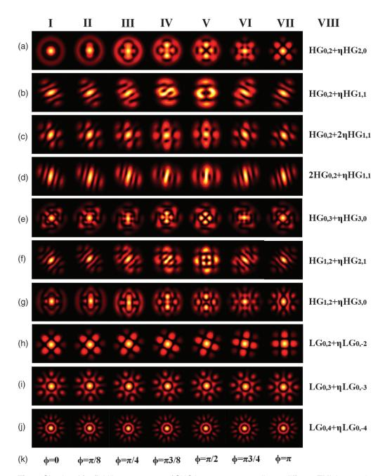
**Fig. 4** Simulated far-field beam patterns of SHG beams corresponding to different TML beams. In column VIII, the TML beams' equations based on Eq. (1) are given. In rows (a) to (g) and rows (h) to (j), different far-field patterns of SHG beams of transverse mode locking states with two HG and LG modes are given, respectively. Here,  $\eta = \exp(i\phi)$ . In row (k), the exact values of the locking phase difference  $\phi$  are given.
