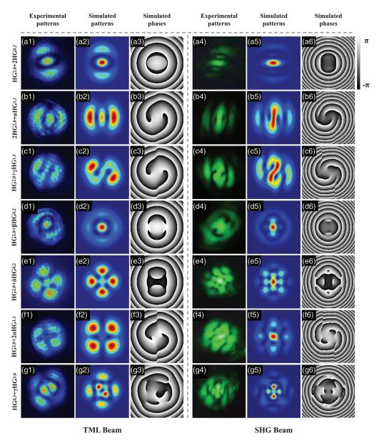
**Fig. 8** The experimental and simulated results for the SHG of TML beams that are composed of  $HG_{m,n}$  modes. The exact combinations of basic modes for each TML state are shown on the left side of each row. Here,  $\alpha = \exp(i\pi/2)$ ,  $\beta = \exp(i\pi/4)$ ,  $\gamma = \exp(i3\pi/8)$ , and  $\delta = \exp(i3\pi/4)$ .
