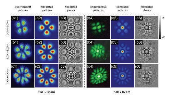
**Fig. 7** The experimental and simulated results for the SHG of TML beams that are composed of  $LG_{0,1}+LG_{0,-1}$  modes. (a)–(c) The combinations are  $LG_{0,2}+LG_{0,-2}$ ,  $LG_{0,3}+LG_{0,-3}$ , and  $LG_{0,4}+LG_{0,-4}$ , respectively. (a1)–(c1) and (a4)–(c4) Experimentally measured far-field beam patterns of TML beams and SHG beams. (a2)–(c2), (a3)–(c3) and (a5)–(c5), (a6)–(c6) are the corresponding simulated far-field patterns and phases.
