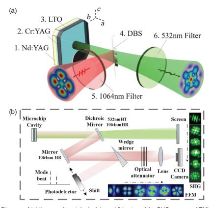
**Fig. 6** Diagram of (a) the experimental principle and (b) setup of the SHG process of TML beams. In panel (a), 1: Nd:YAG microchip; 2: Cr:YAG microchip; 3: LTO, LiTaO $_3$  microchip; 4: DBS, dichroic beam splitter; 5: 532 nm filter; 6: 1064 nm filter; and a, b, c represent the crystallographic axes; c is also the optical axis. (b) The experimental setup and some beam patterns of both the fundamental frequency and SHG beams.
