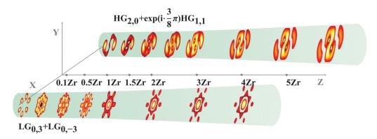
**Fig. 5** Variations of two SHG beam patterns of TML beams in the near field. The upper one is the SHG beam of the TML beam of HG<sub>2,0</sub> +  $\exp(i \cdot 3\pi/8)$ HG<sub>1,1</sub>, and the lower one is the SHG beam of TML beam of LG<sub>0,3</sub>+LG<sub>0,-3</sub>.
