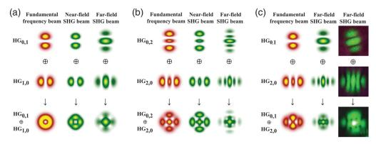
**Fig. 2** The mode compositions in (a), (b), and (c) are  $HG_{0,1} \oplus HG_{1,0}$ ,  $HG_{0,2} \oplus HG_{2,0}$ , and  $HG_{0,1} \oplus HG_{2,0}$ . Here,  $\oplus$  represents the incoherent superposition of the modes. The first and second rows are far-field patterns of two basic HG modes and the third row is the direct intensity superposition of the above two rows.
