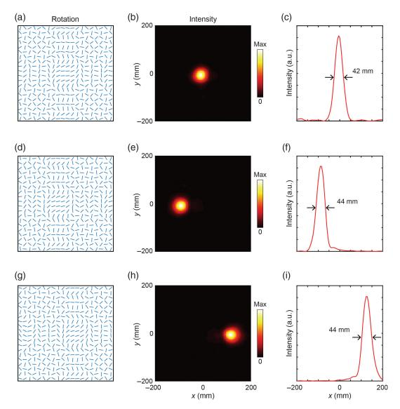
**Fig. 3** Realization of metalensing. (a), (d), (g) Required rotation profiles to realize different metalens operations for RCP waves. (b), (e), (h) Measured electric field intensities ( $|R_{rr}|^2$ ) at 7 GHz on the focal plane. (c), (f), (i) Horizontal cuts of the metalens focal spots, with FWHMs = 42, 44, and 44 mm, respectively.
