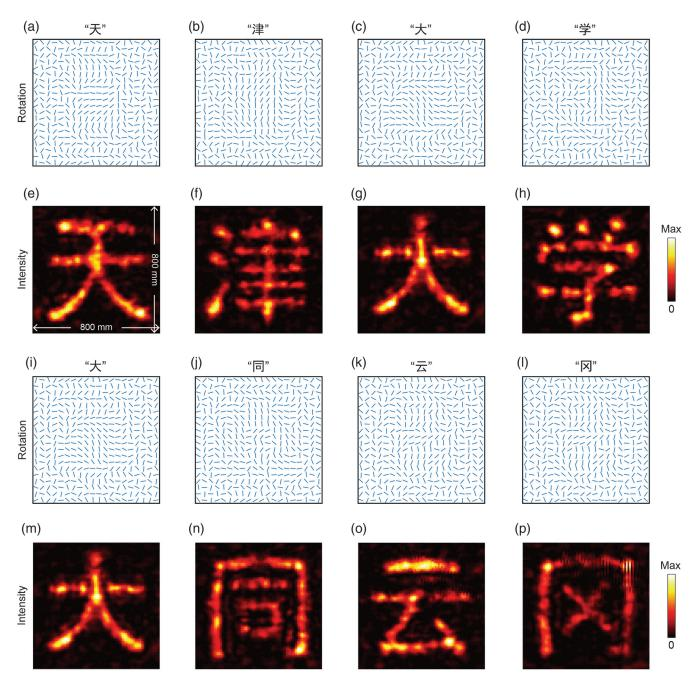
**Fig. 5** Holographic imaging. (a)–(d), (i)–(l) Required rotation profiles to generate holographic images of Chinese characters "天津大学" (Tianjin University) and "大同云冈" (Datong Yungang), respectively. (e)–(h), (m)–(p) Corresponding measured electric field intensities ( $|R_{rr}|^2$ ) of holographic images obtained at z = 600 mm.
