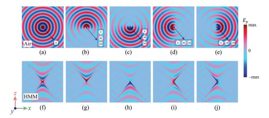
**Fig. 2** (a) Radiation patterns for a simple point dipole in air, where the EM waves can propagate along all directions. (b)–(e) Unidirectional propagation from the Huygens metasource in air. (f) Radiation patterns for a simple point dipole in HMM, where the EM waves propagate mainly along the four channels with high-*k* modes. Panels (g)–(j) are similar to (b)–(e) but for unidirectional propagation of the Huygens metasources in an HMM.
