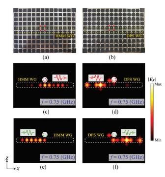
**Fig. 8** (a) Experimental schematic of a circuit-based hyperbolic waveguide. Measured near-field distributions of  $|E_y|$  for (c) counterclockwise and (e) clockwise spin metasources. Panels (b), (d), and (f) are similar to (a), (c), and (e), but for the circuit-based normal waveguide.
