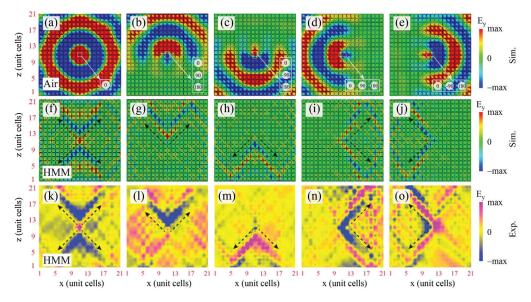
**Fig. 5** (a) Simulated point dipole radiation patterns in the circuit-based normal medium. The EM waves can propagate along all directions. (b)–(e) Unidirectional propagation of the Huygens metasources in a circuit-based normal medium. Panels (f)–(j) correspond, respectively, to (a)–(e) but for the simulated radiation patterns in the circuit-based HMM. Panels (k)–(o) correspond, respectively, to (a)–(e) but for the measured radiation patterns in the circuit-based HMM.
