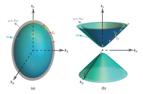
**Fig. 1** Various 3D IFCs for (a) a closed ellipsoid and (b) an open hyperboloid when the frequency increases from  $\omega$  to  $\omega + \delta \omega$ . The energy flows in the *x*, *y*, and *z* directions are marked using red, pink, and yellow arrows, respectively.
