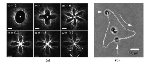
**Fig. 25** Optical trapping with complex optical patterns. (a) Experimentally generated beam patterns with different modes. (b) Two particles being guided along the trajectory shown by the dotted line. Adapted from Ref. 142
