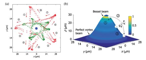
**Fig. 40** Perfect vortex traps in vacuum. (a) Particle trajectories with different topological charges  $\ell = 3$ , 10, and 30 for blue, green, and red crosses, respectively. Circled numbers indicate the order of the walked path when  $\ell = 30$  (red crosses). (b) Topography of the measured perfect vortex and Bessel beams ( $\ell = 15$ ) around the beam axis ( $x = y = 0 \mu m$ ) with a schematic of particle motion. Adapted from Ref. 202.
