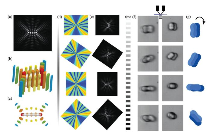
**Fig. 20** Optical trapping of nonspherical particles. (a) Mathieu beam with m = 4. (b) 3D intensity distribution. (c) Particles orientation within transversal intensity distribution. (d) Rotating hologram and (e) corresponding Mathieu beam. (f) Time-lapse images of trapped particles depending on the orientation of the Mathieu beam and (g) their corresponding schematics. Adapted from Ref. 125.
