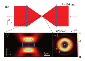
**Fig. 41** Trapping of nanodiamonds with linearly polarized  $LG_{03}$  beams. (a) Schematic of the dual beam trap. (a) Geometry of the trap relative to a nanodiamonds-core (core radius r = 100 nm) coated with a silica shell (shell radius  $R = 1 \mu$ m) (b) from the side and (c) axial views, respectively. Adapted from Ref. 112.
