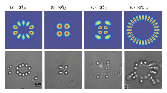
**Fig. 22** Micromanipulation with IG beams. The top row shows the transverse intensity patterns of the beams, while the bottom row shows trapped microparticles with the corresponding beams. (a)  $IG_{5,5}^o$  mode. (b)  $IG_{2,2}^o$  mode with four columns of particles stacked along its beam axis. (c)  $IG_{4,2}^o$  mode where the four central petals close to each other show no stable traps. (d)  $IG_{14,14}^e$  mode with particles trapped at certain locations. Adapted from Ref. 132.
