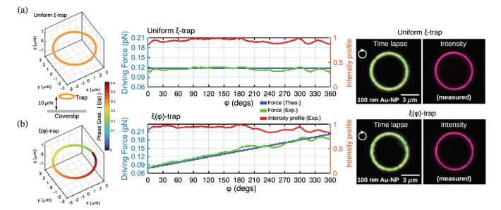
**Fig. 38** 3D trapping and transporting of metal nanoparticles. (a) Left: ring trap with uniform phase gradient. The inset shows that the location of the trap is 10  $\mu$ m from the chamber wall (coverslip). Middle: theoretical and experimental estimated optical propulsion force along the ring of the trap. Right: the time-lapse image of the nanoparticles in the ring trap. (b) Same as those in (a) but for tailored phase gradient. Adapted from Ref. 152.
