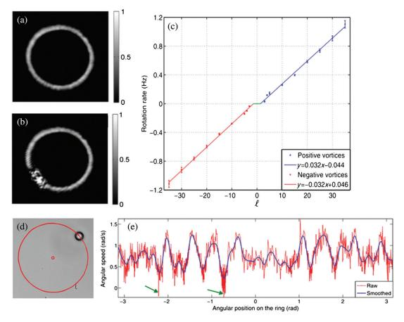
**Fig. 19** (a) A perfect vortex beam with  $\ell = 25$  and (b) the beam with the scattered light from a single trapped particle. (c) Linear relationship between the particle rotation rate and the integer topological charge. (d) Snapshot of a trapped particle rotating around the circumference of a perfect vortex beam indicated by the red circle. (e) Angular velocity of the particle as a function of its angular position. Adapted from Refs. 123 and 124.
