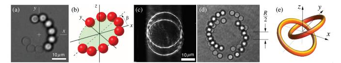
**Fig. 28** Optical trapping and transporting of microparticles along 3D parametrized trajectories. (a) Particles trapped along a single ring in 3D. (b) Schematic representation of (a). (c) Experimental intensity distribution of two tilted ring traps with opposite inclination. (d) Colloidal silica spheres trapped in the two rings of (c). (e) Schematic 3D representation of the knotted rings of (c) and (d). Adapted from Ref. 147.
