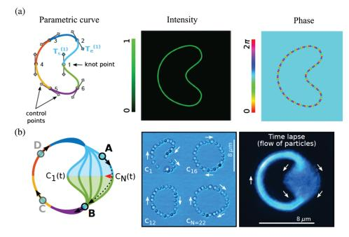
**Fig. 31** Example of a Beziér parametric curve and its application to reconfigure in real-time the trajectory of microparticles. (a) Construction of a parametric curve using (left) Beziér splines, (middle) intensity, and (left) phase of a laser beam following this parametric curve. (b) Example of real-time reconfiguration of the curve shown in (a) and its application in a real-time reconfigurable optical trap (middle). Adapted from Ref. 151.
