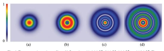
**Fig. 4** Transverse intensity profiles of LG modes with (a)  $LG_0^0$ , (b)  $LG_0^1$ , (c)  $LG_2^0$ , and (d)  $LG_2^2$ . The color denotes the normalized intensity distribution.
