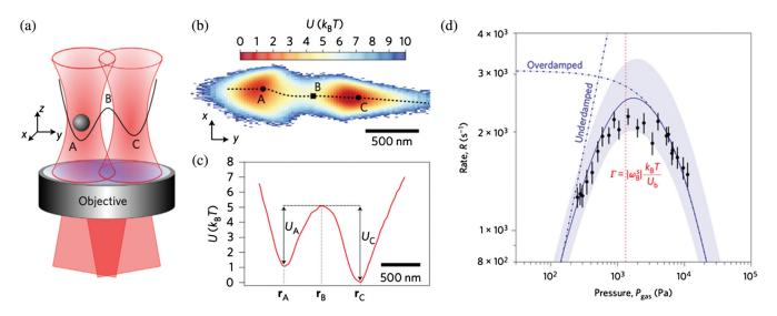
**Fig. 42** Testing Kramers turnover with a double-well potential. (a) Two focused infrared beams forming two potential wells (A and C) linked by a saddle point B. (b) Potential profile in the transverse (x - y) plane, where the dotted line represents the minimum energy path. (c) Potential energy profile with energy barriers  $U_A$  and  $U_c$  at A and C. (d) Kramers turnover rate depending on gas pressure. Adapted from Ref. 209.
