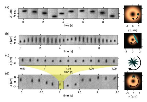
**Fig. 13** Optical trapping and rotations in counterpropagating circularly polarized LG beams of silicon nanowires aligned (a) parallel and (b) perpendicular to the beam propagation axis, where orbiting and orbiting-reorientation are shown, respectively. The simultaneous spinning and orbiting of a shorter nanowire is shown in (c) and (d). Adapted from Ref. 111.
