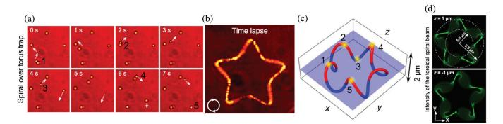
**Fig. 30** Optical trapping with 3D toroidal-spiral beams. (a) Time-lapse images of trapped microparticles moving along the beam over 7 s, which results in (b) a decagon trajectory. (c) 3D schematic representation of the toroidal-spiral curve, where the color scheme indicates the axial *z* position of the curve. (d) Intensity profiles of the toroidal beam at two different axial planes. Adapted from Ref. 149.
