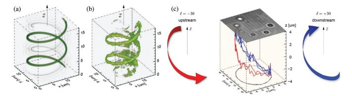
**Fig. 27** Optical manipulation with 3D solenoid beams propagating parallel to the *z* axis. (a) Theoretical and (b) experimental profiles of the beam in 3D. (c) Experimental trajectories of trapped particles transported downward ( $\ell = +30$ ) or upward ( $\ell = -30$ ) along with the helical intensity profile in the optical solenoid beam. Adapted from Ref. 146.
