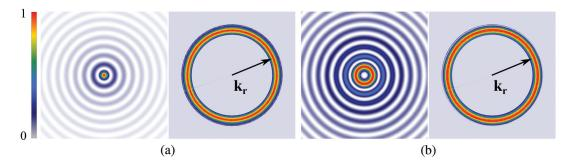
**Fig. 5** Transverse intensity profiles of Bessel beams and its Fourier transform with (a)  $\ell = 0$  and (b)  $\ell = 1$ . The color denotes the normalized intensity distribution.
