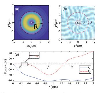
**Fig. 14** Anomalous motion of a particle trapped in strongly focused high-order LG beams. (a) The intensity profile of the LG beam with topological charge 3. (b) The plot of the distribution of the radiation force exerted on the trapped particle for different center-of-mass radii. (c) The radial (blue line) and azimuthal (red broken line) components of the radiation force for different radii of the trapped particles. Adapted from Ref. 113.
