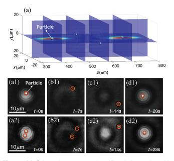
**Fig. 17** (a) Schematic representation of optical trapping with frozen waves in multiple parallel planes. Sequence of  $(a_1)$ – $(d_1)$  one and  $(a_2)$ – $(d_2)$  two microparticles (orange circle) trapped at different transverse planes along the propagation direction. Adapted from Ref. 120.
