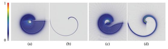
**Fig. 10** Intensity distribution of an HC beam from numerical simulations. (a), (c) The near-field intensity distribution; (b), (d) the far-field. (a), (b) K = 0; (c), (d) K = 1. In all cases,  $\ell = 50$ . The color represents the normalized intensity distribution.
