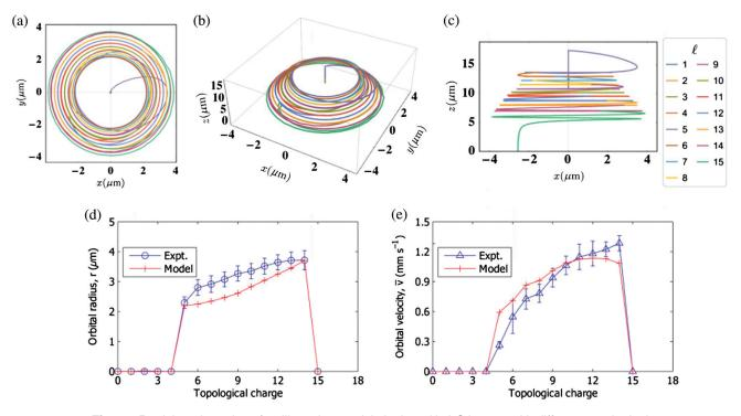
**Fig. 39** Particle trajectories of a silica microparticle levitated in LG beams with different topological charges. (a)–(c) Numerical simulations for  $\ell$  from 1 up to 15. (d), (e) Measured versus calculated orbital radius and velocity as a function of  $\ell$ . Adapted from Ref. 201.
