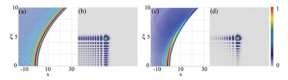
**Fig. 8** Airy beam profiles. (a) Parabolic trajectory and (b) transverse intensity profile of an Airy beam with infinite energy compared with those of a finite energy Airy beam in (c) and (d). The color represents the normalized intensity distribution.
