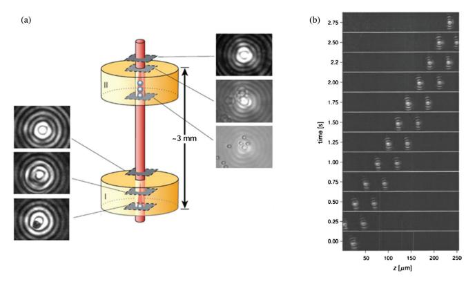
**Fig. 16** Optical trapping with Bessel beams. (a) Trapping of multiple particles at different optical planes. Adapted from Ref. 68. (b) Trapping and delivering of two particles using a sliding Bessel standing beam. Adapted from Ref. 118.
