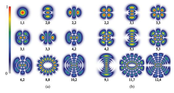
**Fig. 9** Transverse intensity distribution of low-order (a) even and (b) odd IG modes with  $\epsilon = 2$ , z = 0, and  $\omega_0 = 1$  mm. The color represents the normalized intensity distribution.
