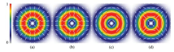
**Fig. 11** Intensity and polarization distribution of the fundamental cylindrical vector beams. (a) Radial, (b) hybrid odd, (c) azimuthal, and (d) hybrid even modes. The color represents the normalized intensity distribution, while the lines are associated with the polarization orientation of the electric field.
