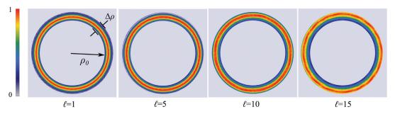
**Fig. 6** Transverse intensity distribution of perfect vortex beams with topological charge  $\ell = 1, 4, 10$ , and 15. Here,  $\rho_0$  is the radius of the ring-like intensity profile and  $\Delta \rho$  its width. Notice that the intensity profile remains constant as  $\ell$  increases. The color represents the normalized intensity distribution.
