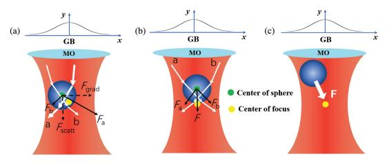
**Fig. 1** Schematic diagram of optical tweezers: (a) when the particle is away from the center of the beam focus, (b) when the particle is slightly above the center of the beam focus, and (c) net force acting on the dielectric sphere.  $F_a$  and  $F_b$  are the forces produced by the refracted rays a and b, respectively.  $F_{\text{grad}}$  and  $F_{\text{scat}}$  denote the gradient force and scattering force, respectively. GB, Gaussian beam; MO, microscope objective.
