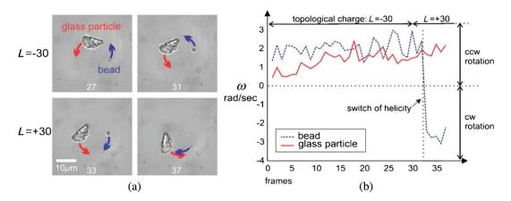
**Fig. 15** Rotation of a polystyrene bead and a glass sliver trapped with an LG mode of  $\ell = \pm 30$ . (a) Sequential images of these particles showing their direction of rotation. (b) Angular velocity of each particle with respect to the topological charge. Adapted from Ref. 114.
