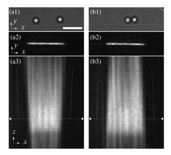
**Fig. 26** Optical trapping with a parabolic phase gradient. Two silica beads (1.5  $\mu$ m in diameter) trapped in (a1) positive and (b1) negative parabolic phase gradients and (a2), (b2) the corresponding beam intensity profiles at the trapping plane. A cross-section of the beams in the *x* – *z* plane, showing (a3) the divergence and (b3) convergence of the phase gradient. Adapted from Ref. 76.
