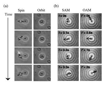
**Fig. 3** Optical trapping of birefringent microparticles that show the transfer of OAM and SAM. (a) The trapped particle is spinning counterclockwise about its own axis (left column) and orbiting clockwise about the beam's axis (right column) separately. Adapted from Ref. 58. (b) The particle rotates around its own axis (left column) and the beam's axis (right column) simultaneously. Adapted from Ref. 59.
