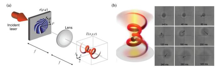
**Fig. 23** Optical manipulation with HC beams. (a) Schematic representation of the setup required for beam generation. (b) Time-lapse images of a microbead trapped and guided along with the maximum intensity of the beam, as illustrated on the left. Adapted from Ref. 133.
