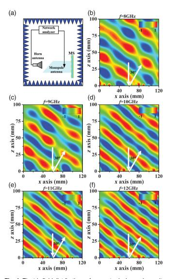
**Fig. 4** Electric field distributions of our meta-device under excitation of  $\hat{x}$ -polarized waves. (a) Experimental setup of the near-field measurement. Measured Re[ $\vec{E}$ ] distributions on the *xoz* plane at the reflection side of our metasurface at (b) 8 GHz, (c) 9 GHz, (d) 10 GHz, (e) 11 GHz, and (f) 12 GHz under excitation of normally incident  $\hat{x}$ -polarized waves. All of the electric field spectra are normalized against the maximum value at each frequency.
