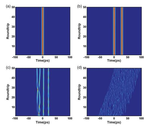
**Fig. 6** The numerical evolutions of the pulses for different  $E_{sat}$  values of (a) 0.06 nJ, (b) 0.12 nJ, (c) 0.4 nJ, and (d) 8 nJ. Reproduced with permission from Ref. 96.
