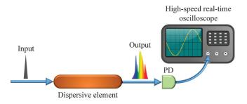
Fig. 8 The optical set-up for the time-stretching measurement method. PD, photodetector.
