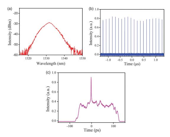
**Fig. 4** The output characteristics of the NLPs: (a) the optical spectrum, (b) the pulse trains, and (c) the autocorrelation trace. Reproduced with permission from Ref. 90.
