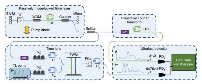
**Fig. 10** Experimental setup of the hybrid measurement method based on time stretching and time lensing. Reproduced with permission from Ref. 152.
