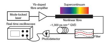
Fig. 1 The optical set-up for RW generation in a supercontinuum system. Reproduced with permission from Ref. 5.
