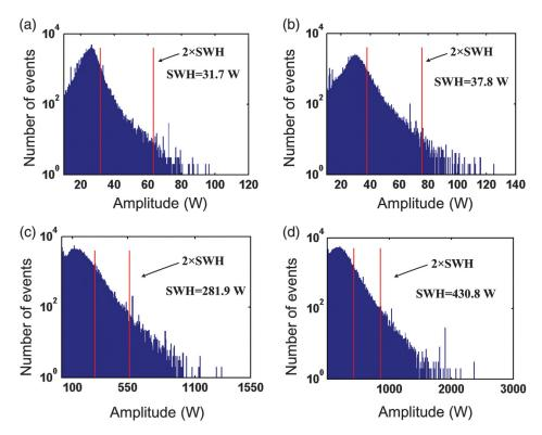
**Fig. 7** The numerical statistical distribution of RWs for different  $E_{sat}$  values of (a) 0.6 nJ, (b) 0.8 nJ, (c) 8 nJ, and (d) 14 nJ. Reproduced with permission from Ref. <u>96</u>.
