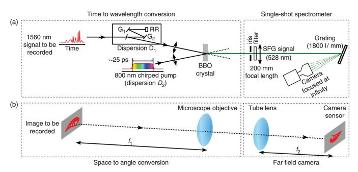
Fig. 9 Time lens for observing RWs: (a) the experimental setup and (b) the spatial analogy. Reproduced with permission from Ref. 145.
