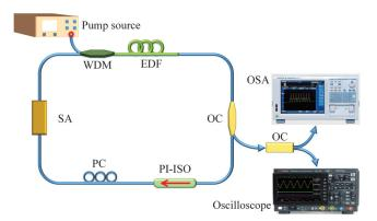
**Fig. 3** A typical schematic diagram of a soliton fiber ring laser operating at 1550 nm based on passive mode locking technique. EDF, erbium-doped fiber; WDM, wavelength division multiplexer; SA, saturable absorber; PC, polarization controller; PI-ISO, polarization-independent isolator; OC, optical coupler; OSA, optical spectrometer.
