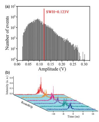
**Fig. 5** (a) The pulse–amplitude statistical distribution histogram for the NLP regimes and (b) the temporal evolution of the localized NLPs. Reproduced with permission from Ref. 90.
