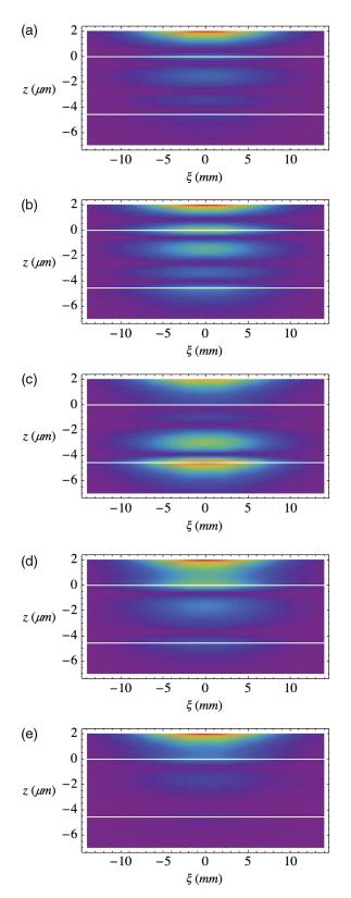
**Fig. 7** The evolution of the electromagnetic field in the slab geometry of Fig. 4(b), near the "ghost resonance," with the incidence angle  $\theta$ : (a) 46.42 deg, (b) 46.44 deg, (c) 46.46 deg, (d) 46.48 deg, and (e) 46.5 deg. The angle  $\phi$ , the system spatial dimensions, and the material parameters are the same as in Fig. 6. Note that the entire sequence (a) to (e) corresponds to the variation of the incidence angle  $\theta$  by <0.1 deg.
