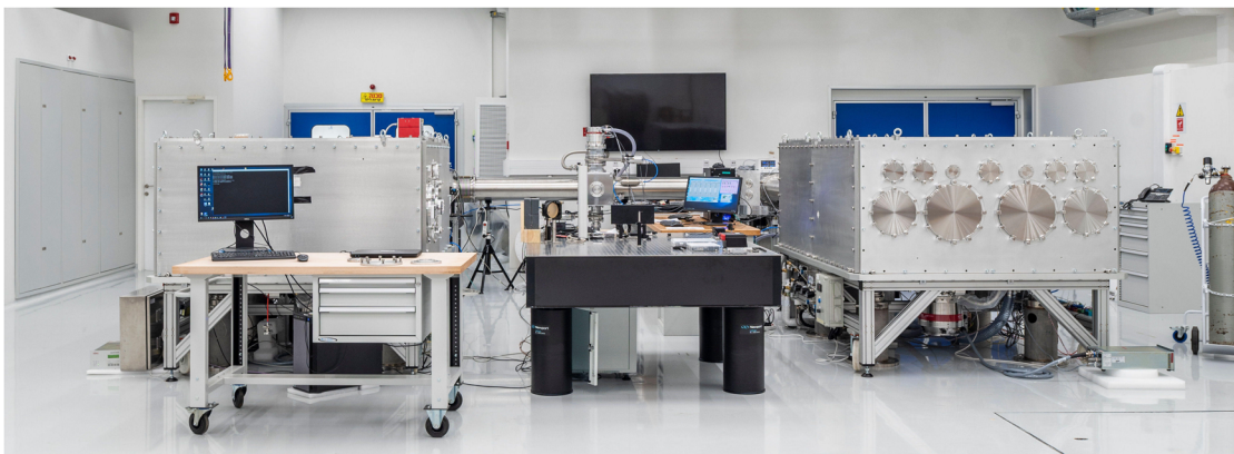
FIG. 4. General view of experimental hall showing the target chambers: electron/x-ray-beam chamber (left); ion-beam chamber (right).
