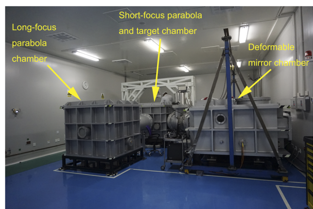
FIG. 1. Target area of SILEX-II laser facility.
