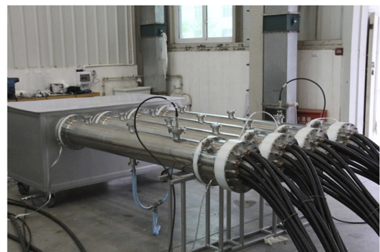
FIG. 5. Photograph of trigger unit, which comprises a mini-Marx, four 7.5\text{-}\Omega/75\text{-ns} water-insulated pulse-forming lines, four laser-triggered gas switches, and 40 75\text{-}\Omega output cables.
