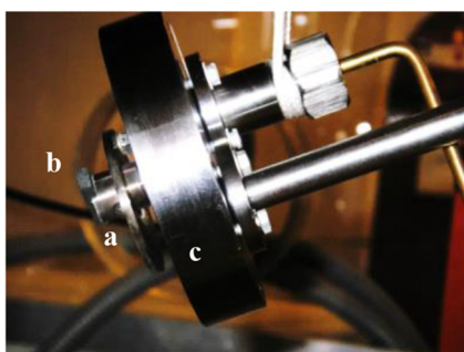
FIG. 2. (a) Specimen holder and (b) a specimen of tungsten attached to (c) the lid of a chamber for use in the PF-6 and Vikhr' devices.
