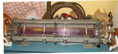
FIG. 7. GOS-1001 laser device capable of working with a pulse of about 50 ns and 20 J in the Q-switched mode.
