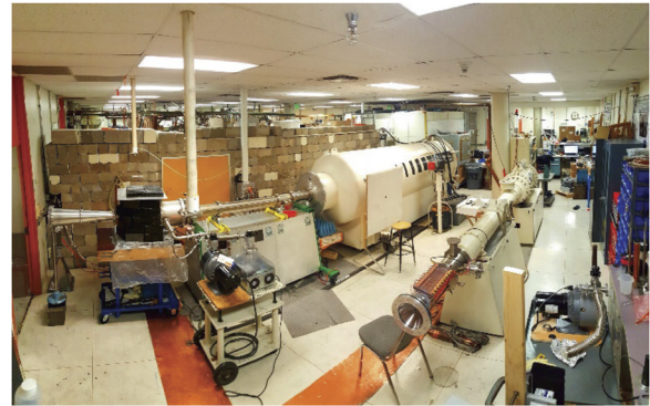
FIG. 19. Photograph of the modified PI-110A accelerator (back) adjacent to the SINUS-6 (front) at UNM.
