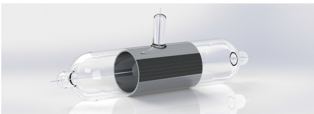
FIG. 2. CAD drawing of the original Hull magnetron.
