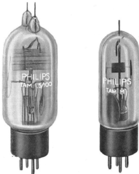
FIG. 7. The early Philips split anode magnetron. Reprinted with permission from Goerth, in Proceedings of International Conference on the Origins and Evolution of the Cavity Magnetron , Bournemouth, UK, April 2010 (IEEE, 2010), pp. 17–22. Copyright 2010 IEEE.
