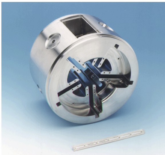
FIG. 14. Tunable rising-sun relativistic magnetron at Physics International. This relativistic magnetron uses plungers moving back walls of three vanes for mechanical tunability. Extraction is through two waveguide ports, one of which is visible. Reprinted with permission from Benford, in Proceedings of International Conference on the Origins and Evolution of the Cavity Magnetron , Bournemouth, UK, April 2010 (IEEE, 2010), pp. 40–45. Copyright 2010 IEEE.
