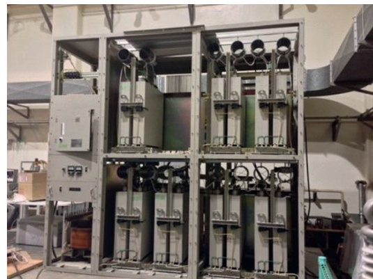
Fig. 3. Picture of the pulsed power generator using the PFN.
