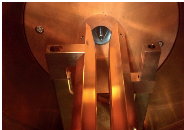
Fig. 10. DPIS injection region. The vertical rods are RFQ's vanes. At the center of the end flange, a stainless steel conical extraction electrode is shown. The electrode is filled by the delivered plasma. The RFQ operates at 100 MHz with 120 kV intervane voltage. The extraction voltage is 60 kV for a 100 mA C^{4+} beam. This RFQ setup is operational at BNL.
