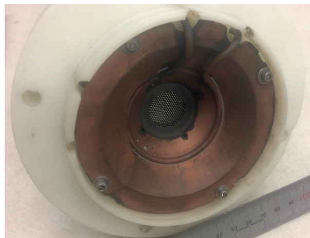
Fig. 9. Multi-hole extraction system. This system has been used to extract hydrogen ions using only 2.8 kV voltage. This grid system provides beam currents more than 100 mA.
