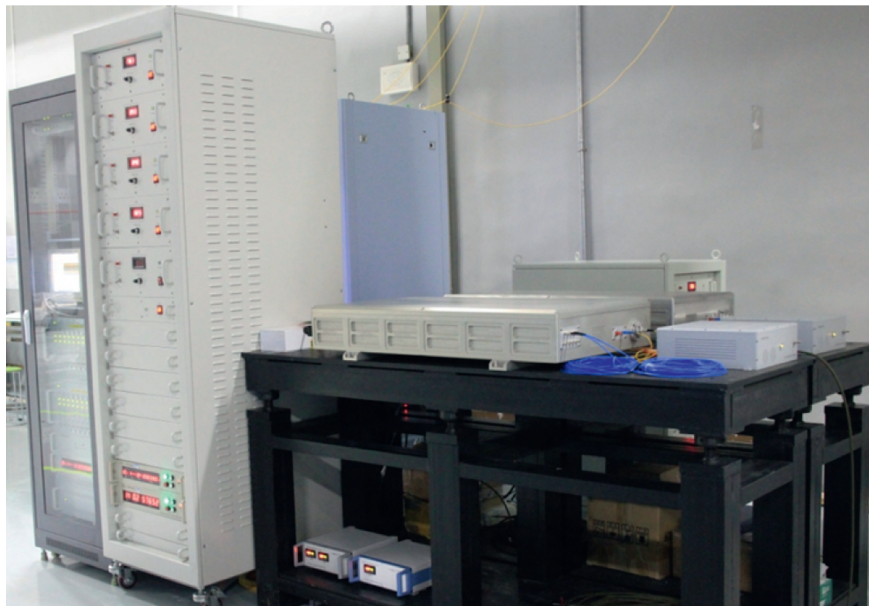
Fig. 7. The laser system for time fiducial and VISAR in SG-III.
