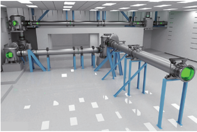
Fig. 11. The initial bypass of the L3 beam transport in the experimental hall E3.
