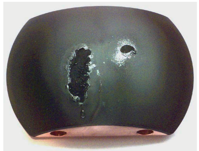
Fig. 16. B_4C -coated test limiter damaged by arcing and melting during the exposure to plasma.
