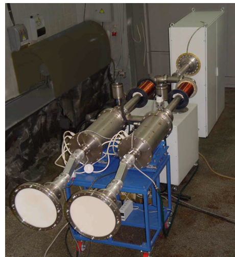
Fig. 7. Two-channel 2 \times 0.3 GW source producing the fourfold power density in the maximum of the interference pattern in the far zone compared to that of each single channel.
