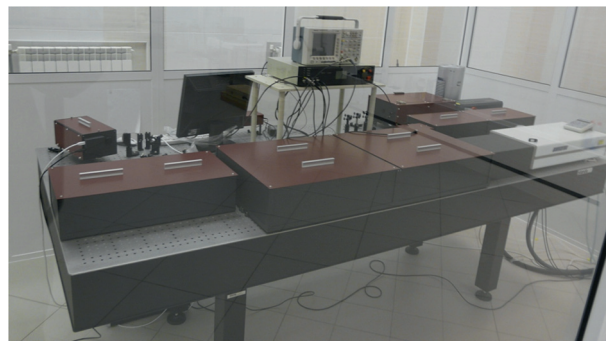
Fig. 10. START-480M Ti:Sapphire starting complex.
