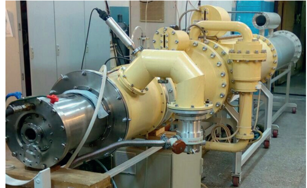
Fig. 6. SINUS-500 with RBWO source operating at 100 pps.
