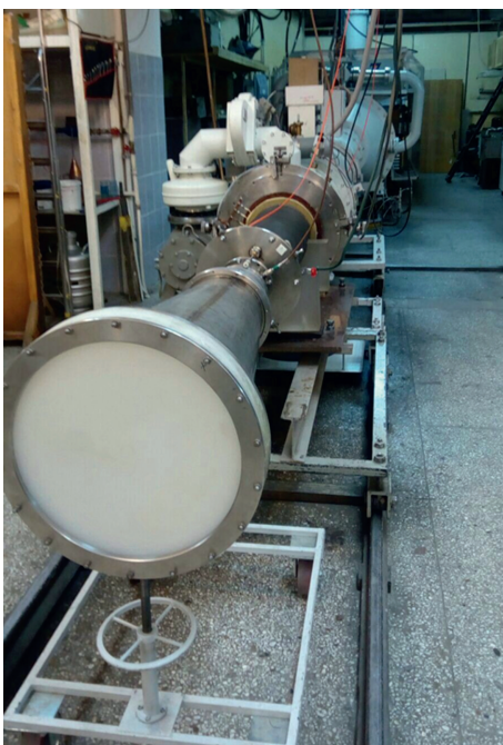
Fig. 5. SINUS-7 with S-band microwave oscillator.
