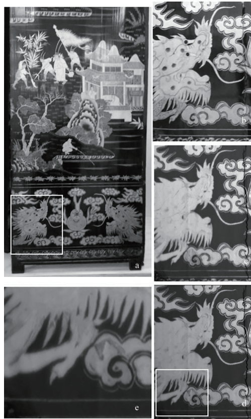
Fig.17 (a) The lacquered screen belonging to the Queen collection. The white square localizes the first scanned area; (b) the first scanned area; (c) THz peak-to-peak image; (d) false color rendering realized by placing the frequency intervals 0.06~0.28 THz, 0.53~0.65 THz, 0.86~0.93 THz respectively into the red, green and blue channel. The white square localizes the anomalous area; (e) relevant detail of the previous image 图 17 (a)女王收藏的漆屏风,白色方块定位了第一个扫描区域;(b)第一个扫描区域;(c) THz 峰峰图;(d) 将频率间隔分别为 0.06~0.28 THz, 0.53~0.65 THz, 0.86~0.93 THz 置于红、绿、蓝通道实现的伪显色。白色方块表示异常区域;(e) 前图的相关细节
