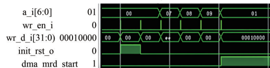
Fig.8 Timing diagram of configuring control status register
