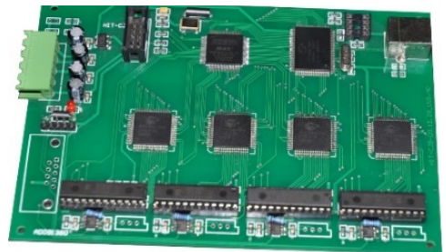
Fig.6 Physical diagram of circuit of weak signal conditioning 图 6 微弱信号调理电路实物图
