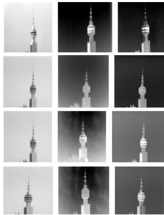
(a) original image (b) infrared image (c) image after inversion Fig.7 Using gray level transformation to realize image conversion 图 7 利用灰度映射法实现图像转换
